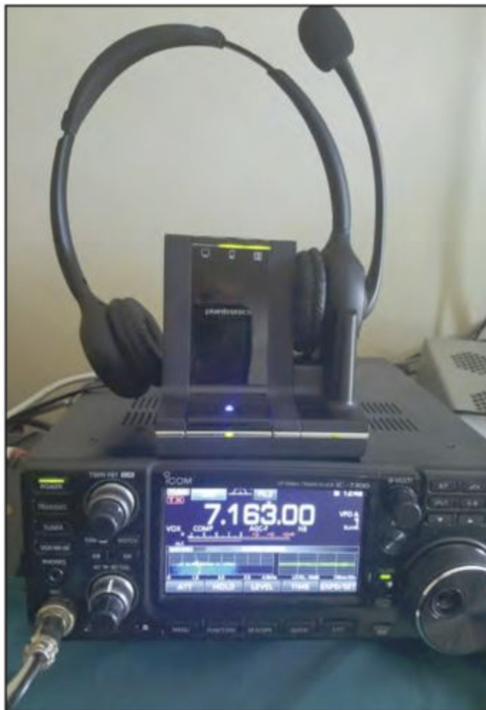
Photo A. The Plantronics Savi W720 wireless headset with WO2 base unit providing multiple connects to a local radio, cell phone, and remote radios. (All illustrations courtesy of the authors)
