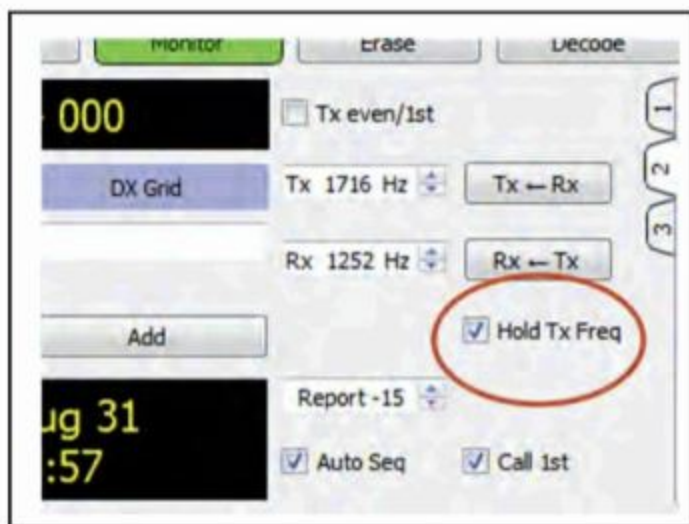
Figure 4. "Hold Tx Freq" checkbox allows you to remain on your transmit frequency while working stations on other frequencies within the FT8 passband.
