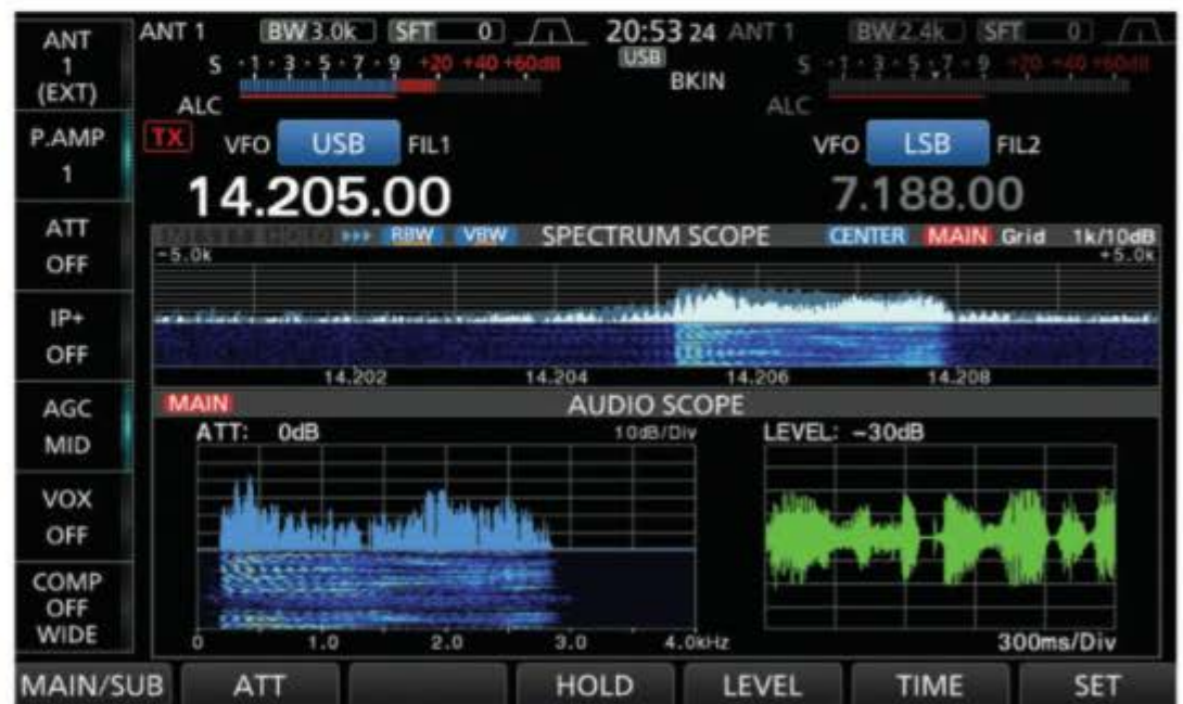
Figure 15. Icom 7610 SDR audio scope display of waveform and spectrum (Credit: Gary White)
