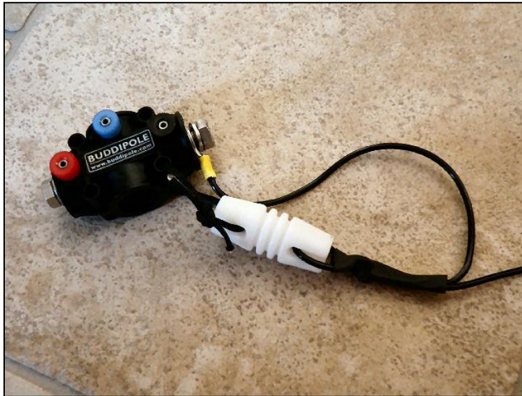
Figure 2. Versa-Tee with Top Insulator and Wire Rope. Bolts on each end are 3/8" dia. x 1/2" long plus lock washer, stainless steel
