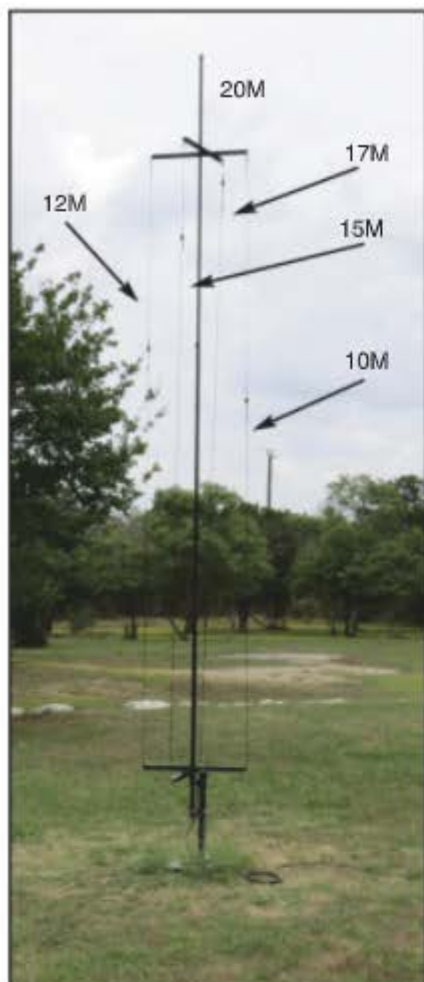
Photo B. After the cross-arms have been attached, wires cut to each additional band are installed between the top and bottom cross-arms.
