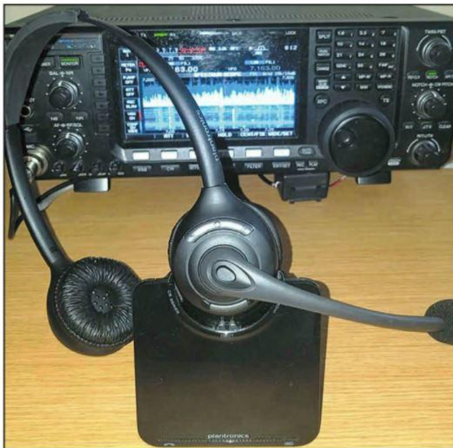
Photo A. The Plantronics wireless headset that the authors modified to let them operate "untethered" from their radios. (All illustrations courtesy of the authors)
