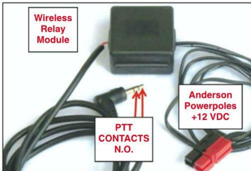
Photo F. Roaming PTT wireless relay module assembly.
