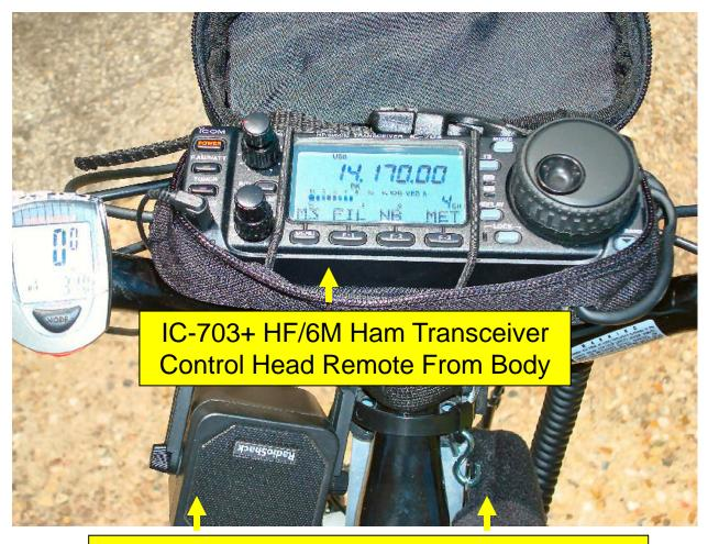
HF/6M Rig's Speaker Hung from Handle Bars Mic Hung from S-hook on Handle Bars
