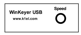
There is one knob that is used to set WKUSB's operational WPM rate. In standalone mode the knob will always control speed. In host mode the speed control may or may not have an affect depending on how the app is configured. Some applications only allow you to change the speed by their own controls and will ignore WKUSB's control.
