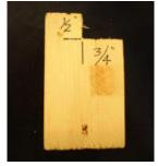
Another useful tool is a 2 x 2 block of wood with a notch in one end. It backs up the tin while center punching the holes. Clamp in a vice and it will make cleanly center punching the holes much easier.
