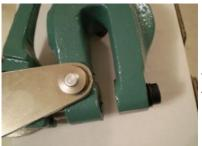
Ensure that the die doesn't protrude into the space between the jaws, see picture on the left.
