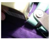
Screw the 1/4" die in the bottom jaw, and insert the 1/4" punch in the top (movable) jaw. If you have the metric version
