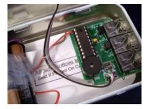
Print the bottom insulator, trim, and place it in the bottom of the tin prior to inserting the board Click the picture to print it at actual size.
