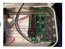
Strip and tin the two remaining wires and solder them into the +5 V and gnd power supply connections at the top edge of the board.
