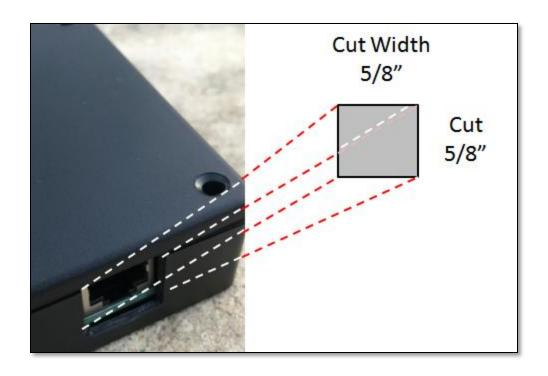
Horizontally Center the Area to Be Cut, 5/8" <u>Width</u> Total. Observe Vertical Cut Out Begins at <u>Top Edge</u> of Box (Not the Lid).
