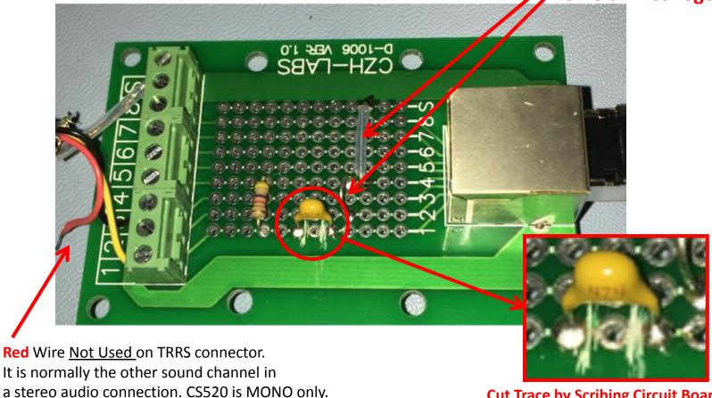
Cut Trace by Scribing Circuit Board
