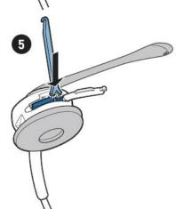
Using the "Y" end of the tool, press the battery backwards
