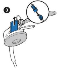
Once the battery is removed, gently disconnect the battery connector;
