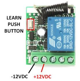
Mode 3 is Time Delay meaning the contacts close when the sender button is pressed momentarily and the relay maintains the closed contacts state until a time delay of 5, 10 or 15 seconds occurs. The time delay is selectable to one of the 3 values determined during programming.
