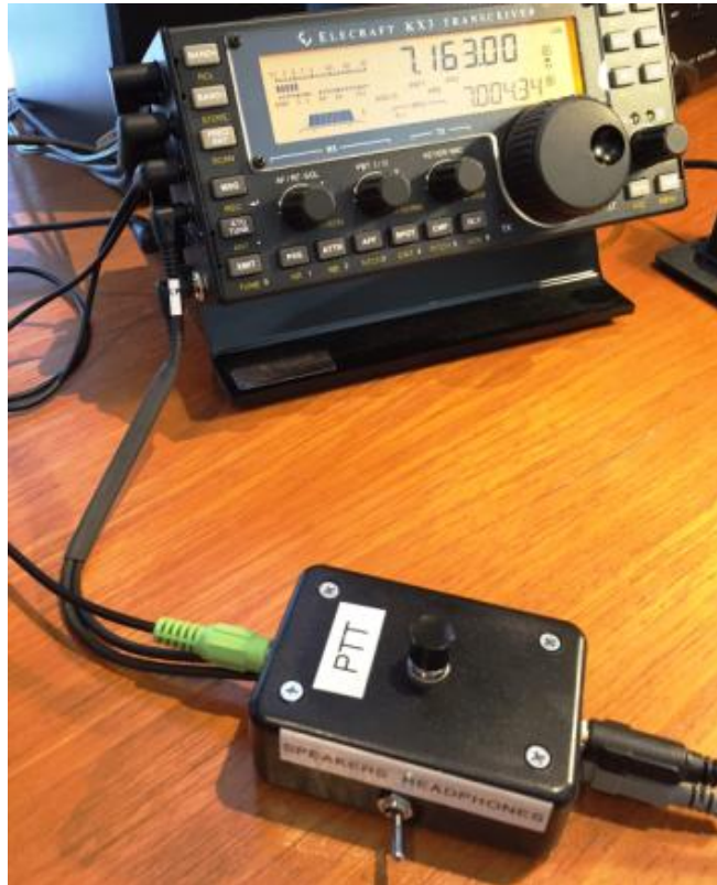
Figure 2. Prototype ASU Connected to KX3 Transceiver Audio Output and Microphone Input
