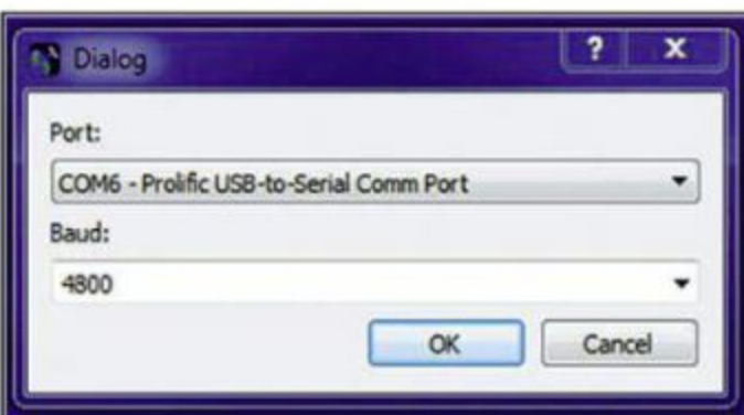
Figure 6. Dialog for Com port settings of the GPS receiver.
