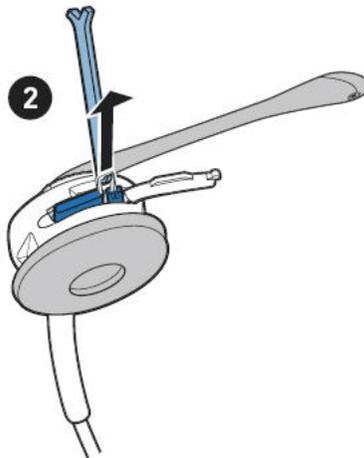
Use the hook end of the tool to hook the battery wires and pull them toward the open battery door until the battery moves out from behind the post.
