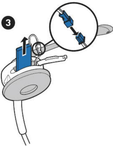
Once the battery is removed, gently disconnect the battery connector;
