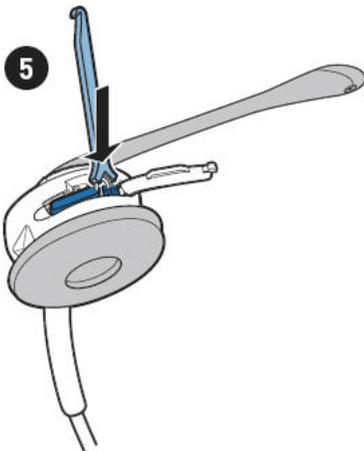
Using the "Y" end of the tool, press the battery backwards
